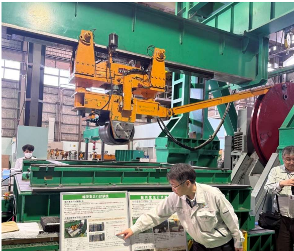
Photo 5 ・ Wheel-load (rolling) test rig for concrete pavement slabs
