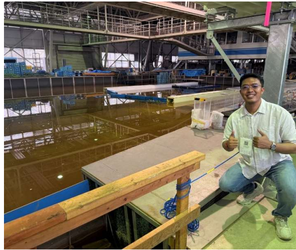
Photo 4 ・ Wave basin used to simulate tsunamis
